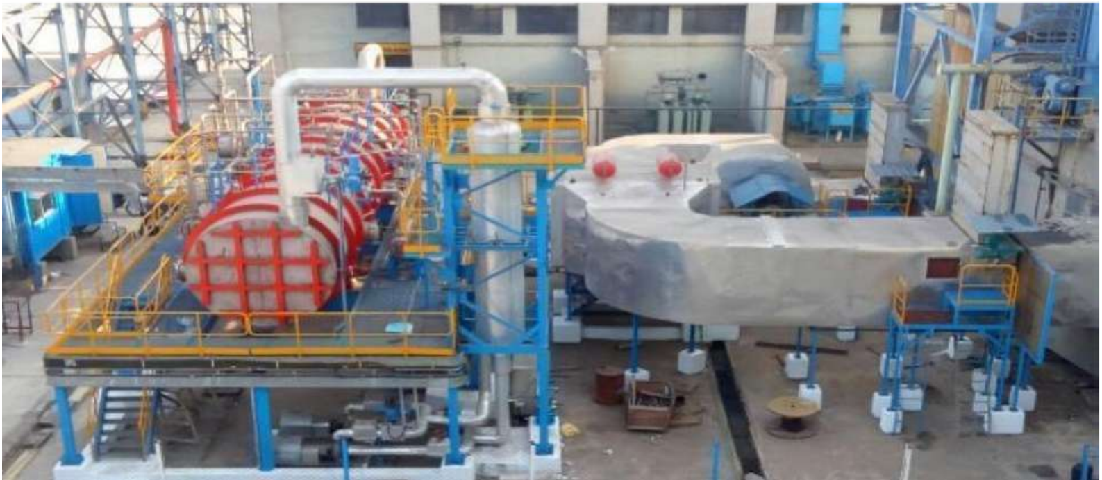
Flue Gas based Sea Water Desalination System
